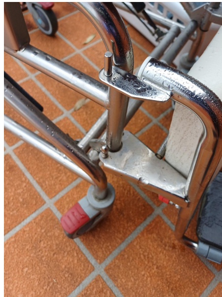
Bathroom and shower mobility equipment showing visible build up of biofilms and mould in crevices, brackets and on flat surfaces.- Pure Wheelchairs
